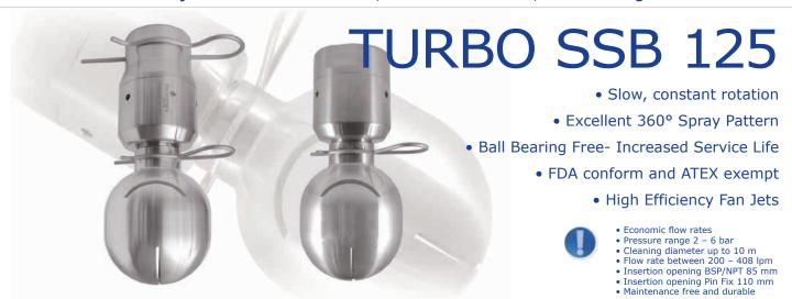
The Turbo SSB 125 is a slowly rotating rotary nozzle. During operation, liquid flowing through it sets the spherical head into a steady braked rotation. In the process, flat jets of liquid with a long range emerge through slots. The slow rotation of the nozzle favours an effective concentrated liquid impact with a high cleaning effect. This achieves a cleaning effect of up to 10 metres in diameter.
