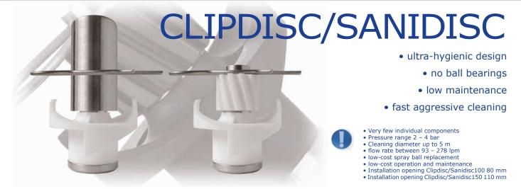
The CLIPDISC/SANIDISC has been developed for many applications where high demands are made on hygiene and product purity. The CLIPDISC is easy to dismantle, meets all regulatory requirements and is also very cost effective. The simple disc design produces complete coverage with cleaning liquid in a swift and aggressive washing process. The cleaning fluid forces a simple disc to rotate rapidly.
